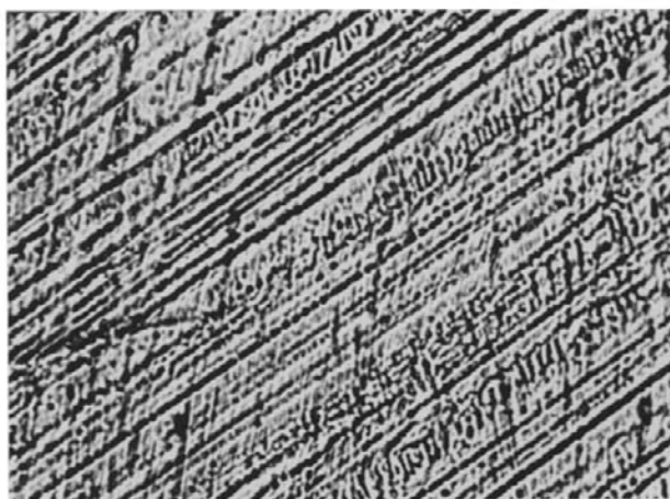
Fig. 8. Microstructure of Ph-PDB eutectic, (magnification, 600×).
